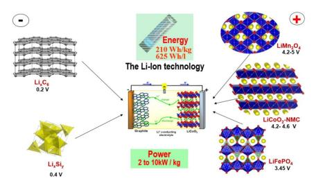
Figure 1. A schematic overview of Li-ion batteries
