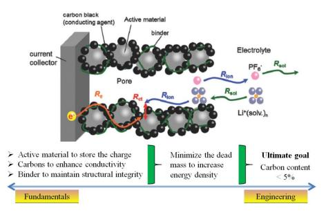
**Figure 2.** A schematic of a porous cathode composite consisting of active material, carbon additive and binder.
