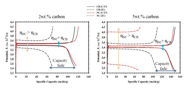
**Figure 5.** Potential versus capacity plots for coin cells cycled at C/17 and 2C rates with LP30 electrolyte.
