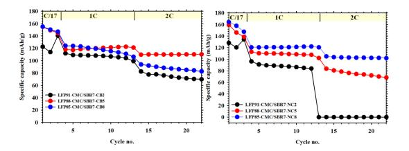
**Figure 4.** Specific capacity versus cycle number for coin cells cycled at C/17, C and 2C rates with LP30 electrolytes.
