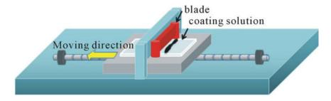
Figure 3. Doctor blade coating of a current collector for Li-ion battery electrodes.
